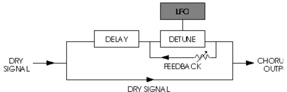
Many variables are available, from varying the speed and depth of the LFO to feeding back part of the signal to make the effect stronger. The Flanger's waveform shape can be either "Normal" or "Inverted". Use the "Inverted" setting for a more dramatic flange effect.
