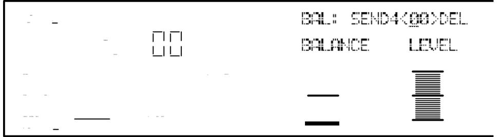
There are only two parameters: Balance and Input Level. This is because in Configuration #1, effect send 4 only has a Delay effect, and not a Pitch effect like the other effect sends do. Quad Knob [1] controls the Balance between the Delay output and the dry effect send signal, while Quad Knob [3] controls the overall input level to the Reverb.
