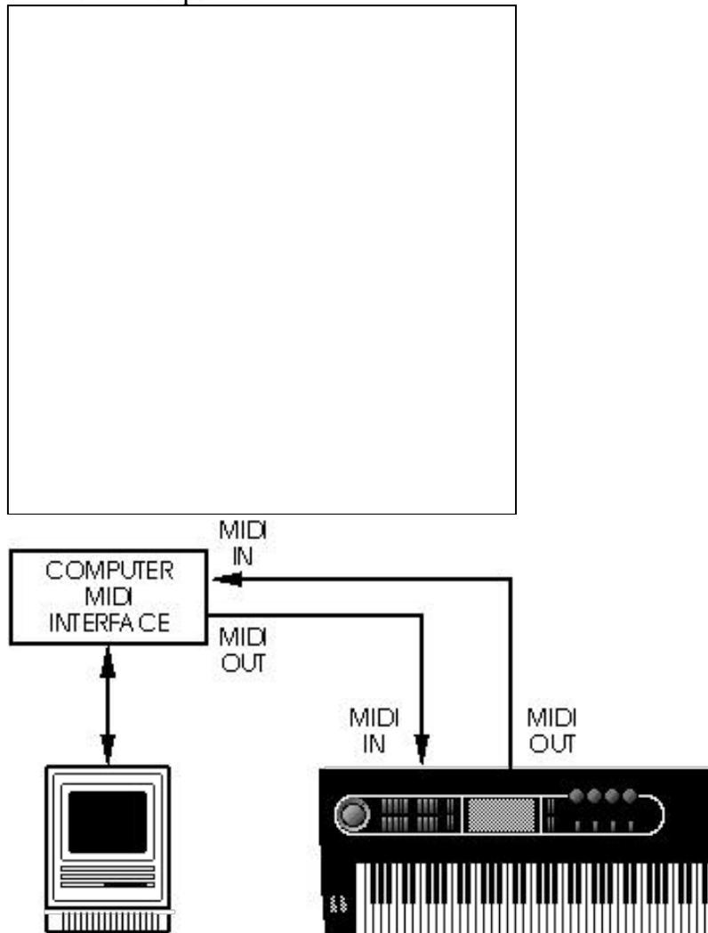
If you are driving other MIDI gear (such as an expander module or MIDI-responsive signal processor), you'll usually drive these from the sequencer if it has additional MIDI outputs. However, you can also use the QuadraSynth Plus's MIDI THRU connector to drive other modules since the Thru carries a replica of what appears at the QuadraSynth Plus's MIDI IN, which is the same as the sequencer's MIDI OUT.
