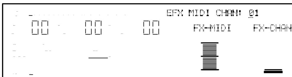
Quad Knob [4] (FX-CHAN) lets you select which Channel (1—16) of the Mix whose Effects Patch you wish to use. If you set the Effect Channel to 1, the Mix will use the Effects Patch used by the Program on Channel 1. The Effect Channel is also used to determine what MIDI channel the Effects Patch will be set to for receiving MIDI controller information for the Modulators (see the Mod section later in this chapter for more on real-time MIDI control).
