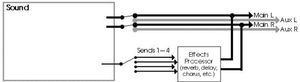
Effects parameters are edited separately from either the Program or the Mix, using Effects Edit Mode (more in Chapter 7). In Program Edit Mode, each of the four sounds in the Program has its own Effect Level control and can be assigned to any one of the four effect buses. Effects settings, Effect Level and Bus information is saved with the Program when you store it back into memory.
