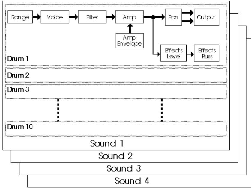
When Drum Mode is enabled, the sound will have fewer parameters for editing. Consequently, not all Function labels will appear in the LCD display as when Drum Mode is turned off. Specifically, the LFOs and all Envelopes (with the exception of the Amp Envelope) are unavailable. In addition, the parameters in most other functions will differ.
