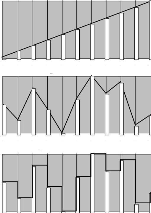
*Tip:* The Tracking Generator can be used to turn a variable control, such as the Mod Wheel or velocity, into a switch by setting all of the points to 0 except for point 10. Only near the maximum input will anything other than 0 come out of the Tracking generator. You can patch the Mod Wheel somewhere else in addition to the Tracking Generator, giving you gradual control of one function with the full range of the Mod Wheel, while switching on a second function only at the top of the wheel.
