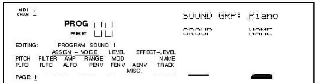
The Assign Voice function is the most fundamental part of Program editing. It is where you choose the particular sample that forms the basis of a sound. To avoid scrolling through long lists of samples (remember, there are 24 megabytes of sounds in here!), sounds are divided into groups. After selecting the group, you then select the sample within the group.
